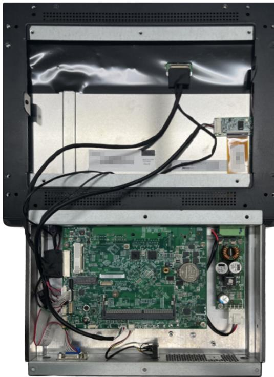
2. Install the memory or M.2 modules carefully, as needed.
